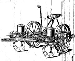
Runner or disc openers, automatic marker (twin disc if preferred) in fact equipment to suit your needs. It's the smoothest combination of time-proved principles you ever saw in a corn planter.
